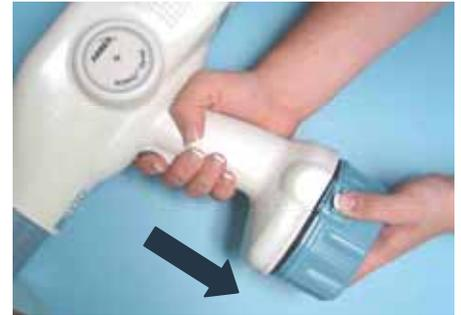
③ Carefully insert a newly charged battery into the base of the NOMAD handle (a properly oriented battery should click into place without force, forcing the battery into position may damage the battery and/or the NOMAD). A clicking sound ensures that the snaps on both sides of the handle bottom are fastened. Make sure the battery is secure by giving it a tug. When a battery is detached, any stored exposure time is erased from memory and has to be reset when the unit is turned on again.
