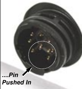
Figure 20B - Recessed Pin
