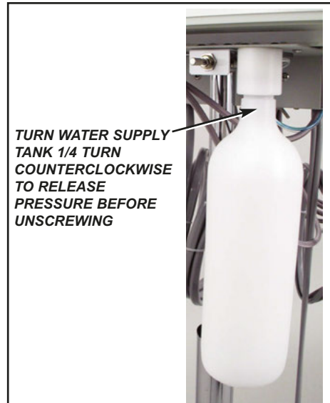
Figure 9 - Water Tank Removal
