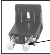
FUSES LOCATED IN VOLTAGE SELECTOR MODULE
