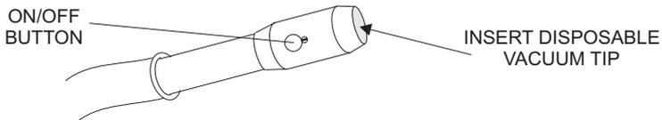
Avoid waste flow-back during use by keeping the ON/OFF button depressed prior to entering the oral cavity and until the hose end has been removed from the patients mouth. Clean the entire hose assembly and waste bottle after each use by evacuating a cleaner/disinfectant through the system and thoroughly scrubbing entire assembly. **CAUTION:** Use only NON-foaming cleansers in the vacuum lines.
